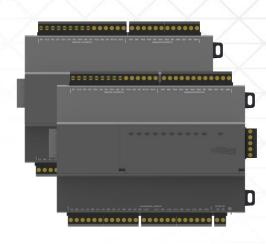
Updated to support 2 IO-R-34 modules and control of both onboard and remote IO with ACE, utilize Edge 10 in more projects and for more applications by enabling critical control of field equipment that require additional IO modules
