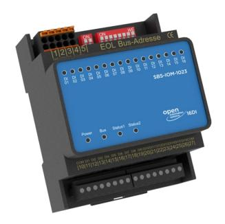
The digital - binary input module **OAS-SBS-IOM-1023** is used for signaling of up to 16 digital messages. These include operating messages, error messages such as frost, filter dirty or fan belt damaged, and status messages such as damper positions.
